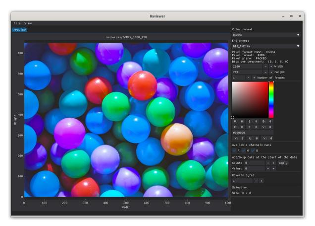
To quickly identify the root of the problem, turn the color channels on and off. When only the red channel is turned on, balls that are blue in reality are shown as very bright:
