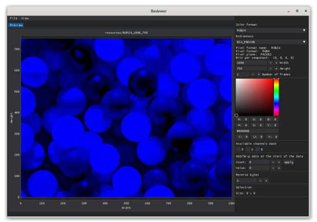
That means that channels R and B are swapped, and the format of our frame is not RGB24 but BGR24.
