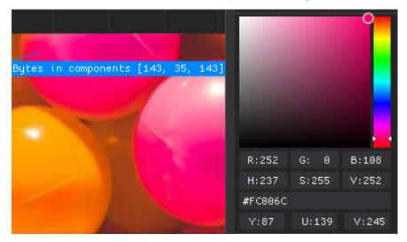
Bytes in components display the channel value in the selected format. You can use this information to determine if the color channel values are correct.
